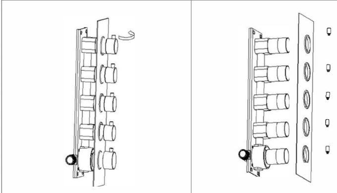
1. Release the handles by unscrewing spigot handles and grub screws according to above directions.
